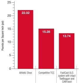
Even when the ToeBoggan footplate is left intact, the FastCast OLS system provides comparable pressure reduction to the competitive TCC.
